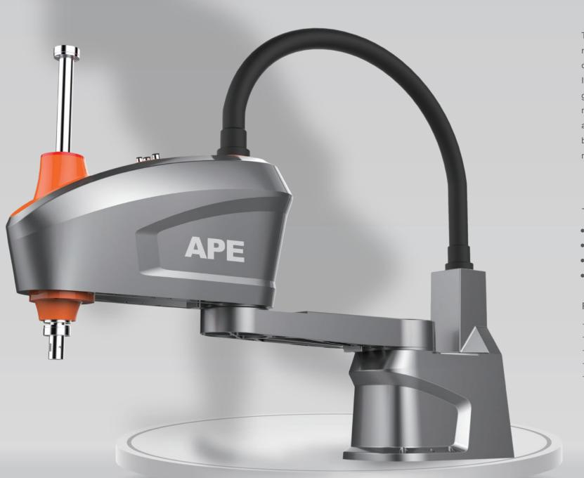
The series of industrial robots are multi joint, multi degree of freedom robots, flexible action, compact structure, easy to install and configure. It has the advantages of short stabilization time, good dynamic performance and high motion repeatability. The body adopts internal wiring, and the joint adopts modular design and assembly. It is easy to maintain and can effectively replace the light manual operation below 6kg.
